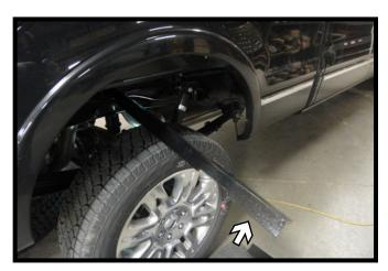
On the passenger side, slide the rear crossmember across the top of the frame towards the rear of the bed hole.
