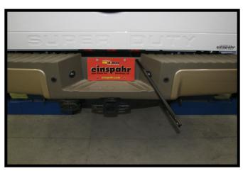
Using the vehicles jack handle tool, remove the spare tire as per vehicles owners manual.
