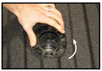
1. Rotate the locking collar to release the latch pawl.
