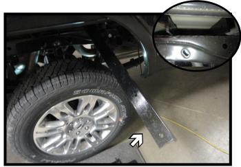
On the passenger side, slide the front crossmember across the top of the frame towards the front of the bed hole.
