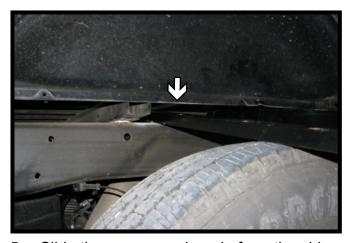
5. Slide the cross members in from the side. Push the flat end in just ahead of the rib. Slide the angle in part way, lift up and bend the rib then finish pushing it in, then bend the rib back. Turn so that the holes are on the lower side, facing down and to the back.
