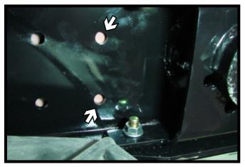
14. Using a 19/32" drill bit, drill the two (2) holes closest to the ball thru the bed. Do this on both sides of the center section.
