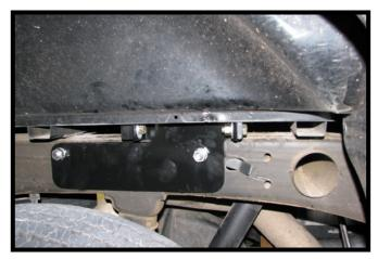
12. Tighten and torque all bolts. First torque the 5/8" bolts. Then torque the outside 1/2" bolts and work in to the 1/2" center section bolts.
