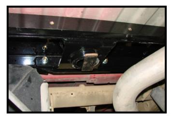
7. On both sides of the center section, bolt the cross members to the center section with the supplied 1/2" hardware. Do not fully tighten hardware.
