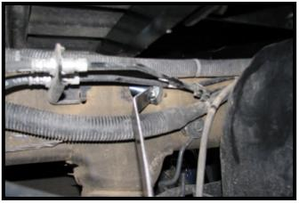
11. Insert the 11"L x 5/8"-11 bolt plate in the opening forward of the fuel tank. Turn the bolt so that it is pointing out. Align with the hole on the outside edge of the frame. Install a 5/8" lock washer and 5/8"-11 hex nut onto the bolt. Do this on both sides of the vehicle.
