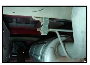
15. Insert the 1/2"-13 u-bolts thru the holes from the topside. Install a 1/2" flat washer, a spring, another 1/2" flat washer and 1/2"-13 lock nut onto each u-bolt stud. Tighten until the washers are touching the spring without compressing it.
