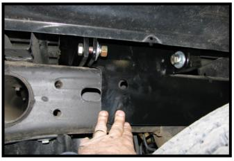
Align the holes at the end of the angle and the rear cross member. Install a 1/2"-13 x 1-1/2" bolt with a 1/2" lock and flat washer. On the front use a 1/2"-13 x 1-1/2" bolt with a 1/2" lock washer and 1/2"-13 nut. Do this on both sides of the vehicle.
