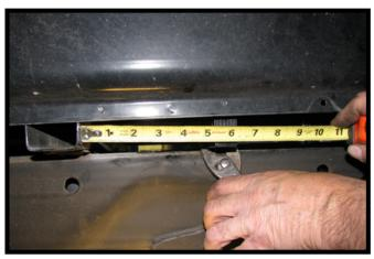
8. On the backside of the bed rib, measure to the 1"x2" cross member. Set to an equal distance on both sides so the hitch is square with the vehicle.
