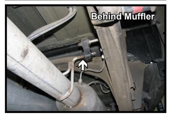
Drop the exhaust by sliding the three
