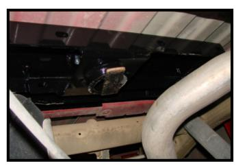
Install the center section, by sliding it in from the backside over the axle then aligning with the hole in the bed. Secure in place.
