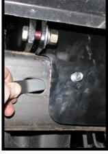
10. Insert a 5"L x 5/8"-11 bolt plate into the front opening. Slide the bolt into the hole and push back so that the bolt comes through the front hole. Install a 5/8" lock washer and 5/8"-11 hex nut onto the bolt. Do this on both sides of the vehicle.
