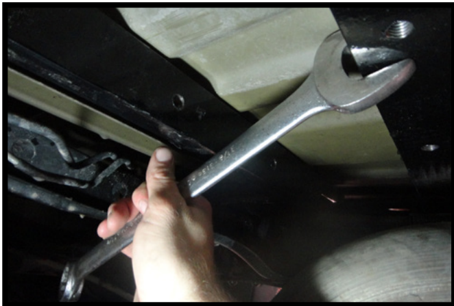
8. Laying the cross members flat, install one end up onto the top of the frame then swing the other end in on the opposite frame. Slide the front cross member forward of the hole and the rear cross member to the rear of the hole.
