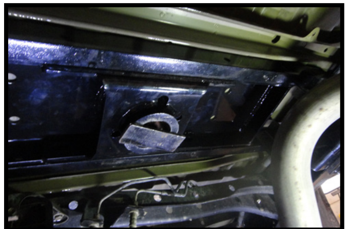
9. Install the center section in between the cross members aligning it to the hole in the bed.
