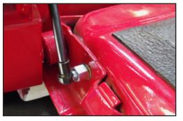
Periodically check the upper and lower mounting locations to insure that parts have not loosened through repeated use. If either mounting location is found to be loose, re-tighten the hardware as needed.
