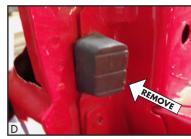
WARNING: If the rubber block is not removed, it will interfere with the shock.
