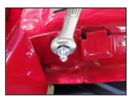
Using a torque wrench to install the ball mount will also insure that the blind nut has been completely installed.
