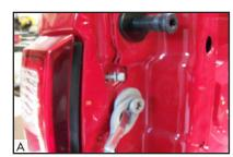
There will still be 2 clips holding the tail light in place. pull the tail light towards the rear of the vehicle to remove it.
