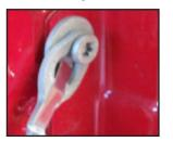
Use a T50 torx socket or the wrench provided to remove the cable bolt.
