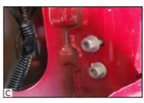
Inside the taillight opening, use an 11mm socket to remove the 2 nuts holding the rubber block in place.
