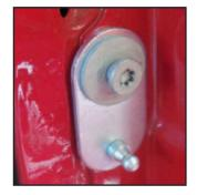
Tighten the bolt with the T50.
