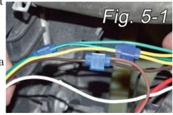
4. Tape all connections using a high-grade electrical tape.
