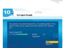
Once accurately pointed, the signal meter will show a signal strength. You'll want to make small adjustments to get the signal as high as possible. Once the signal is peaked, select Done.
