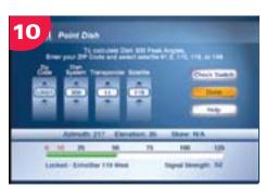
Make sure the satellite is the desired satellite you want to point at. If using Satellite 119 or 110, use **Transponder 11**. If using Satellite 129, use **Transponder 19**.
