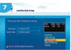
In the box it now gives you an AZIM (Azimuth Angle) and ELEV (Elevation Angle). These are the pointing angles you will need when you go to point the dish.
