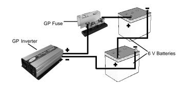
\*Installation using two 6 volt batteries.
