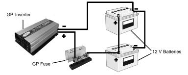
\*Installation using two 12 volt batteries.
