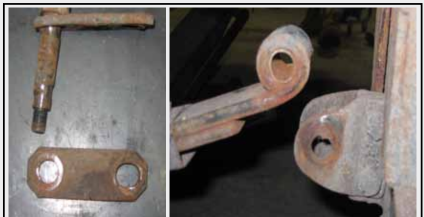
Old shackle assembly and disassembled equalizer.
