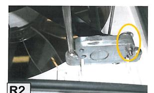
If there are no Brackets, reinstall the screws and washers to hold the Operator to the MaxxFan Base.
