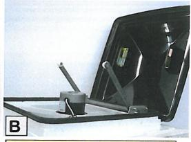
Un hook Lifter Arms from Lid so Lid can fully open to allow access to top of MaxxFan. Be sure to save the Nylon Bushings on the end of the Lifter Arms.
