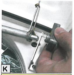
Pull Operator off of Lifter Arm.
