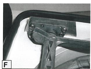
Remove the four Screws that hold the Operator Mechanism to the bracket Save all screws & washers
