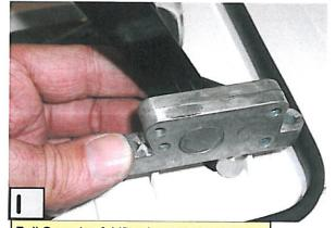
Pull Operator & Lifter Arm up away from Bracket and Remove Operator from end of Lifter Arm shaft. Proceed to Step J to Install Replacement Operator.
