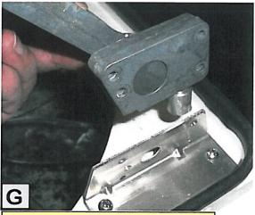
Pull Operator & Lifter Arm up away from Bracket and Remove Operator from end of Lifter Arm shaft.
