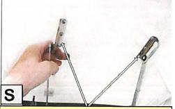
Open lid as needed to reattach Lifter Arms to Lid. Be sure to reinstall Nylon Bushings if present.
