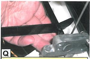
Position the Lifter Arm horizontal (parallel to RV roof) and slide Operator onto the end of Lifter Arm.
