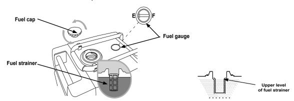
**3.** If fuel is low, with the fuel cap off, pour fuel slowly over the fuel strainer. Do not fill past the upper level of the fuel strainer. Avoid getting dirt, dust or water in the fuel tank.
