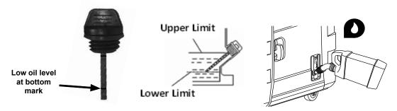
c. After refilling, check the oil level again, and ensure that the oil level is at the top mark on the dipstick.
