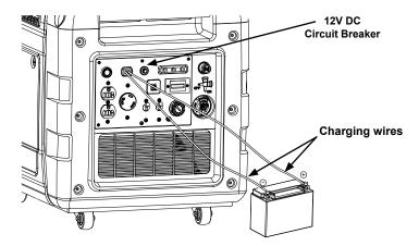
**4.** When charging is complete, disconnect the charging cable from the generator, then disconnect from the battery.
