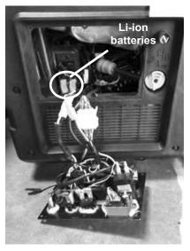
3. Remove the two Li-ion batteries.
