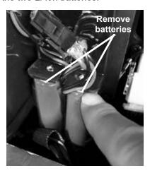
4. Insert two new Li-ion batteries.
