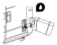
**6.** After refilling, insert the dipstick back into the oil reservoir. (To ensure an accurate reading, do not tighten or screw the dipstick into the reservoir.) Remove it, and ensure that the oil level is at the top full mark on the dipstick.
