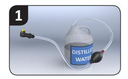
Insert the squeeze bulb filler assembly into a jug of distilled water. Prime bulb by squeezing until it is filled with water.
