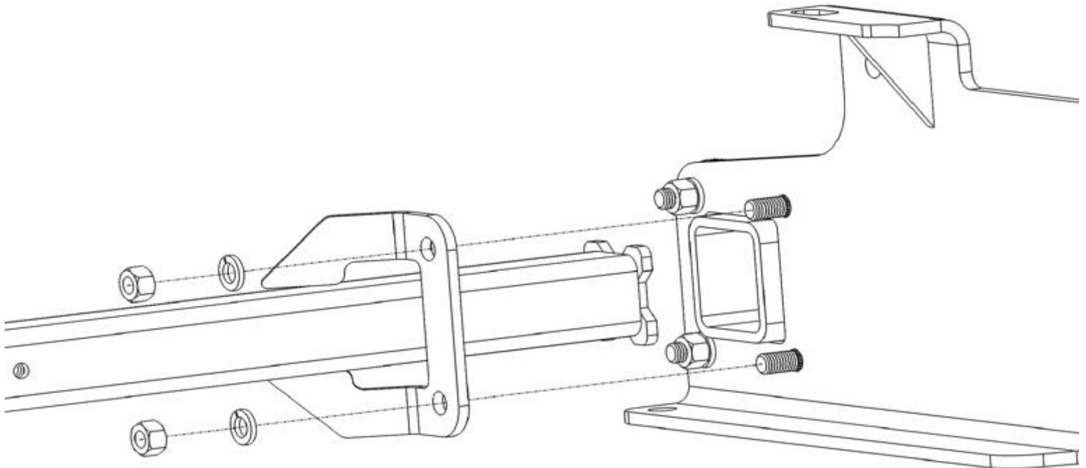
**2.** If there was not at least 1/4" of threads sticking passed the nuts before they were removed, the rib neck bolts will need to be replaced. One at a time, Replace the two Front **Rib Neck Bolt** on the Super Hitch Cross Tube with the provided **1/2"-13 x 1-7/8" Grade 8 Ribbed Neck Bolts**
