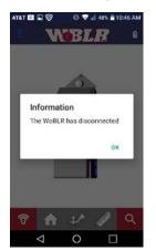
paired and connected WoBLR. You will receive an Information message that the WoBLR has disconnected. The WoBLR will disconnect for several reasons, there is a built in 30 minute shutdown timer that will disconnect you automatically, this is too save battery power. The WoBLR will disconnect If the Bluetooth
