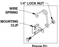
Figure D1: Leveling kit parts.
