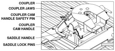
Figure F1: View of Slider Base and Coupler Head assembled.
