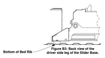
6. Secure the base of the Slider to the truck bed by tightening the 1/2" x 3-1/2" draw-down bolt to 80 ft-lbs, see Figure B4.
