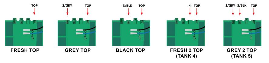
For Tanks 4 - 7 also cut the TOP tab as these examples indicate.
