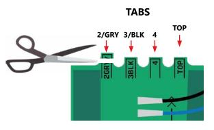
Senders are programmed by cutting off the tabs at the top of each sender to tell it which tank it will be mounted on, or if in a stacked configuration, whether they are on the top or bottom. A pair of scissors or a hole punch can be used to cut the sender tabs.
