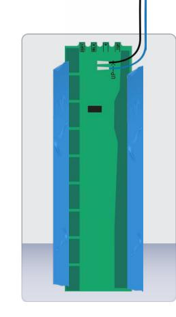
**A CAUTION:** Route wires to the right, away from the senders. The wires indicate the top of the sender.
