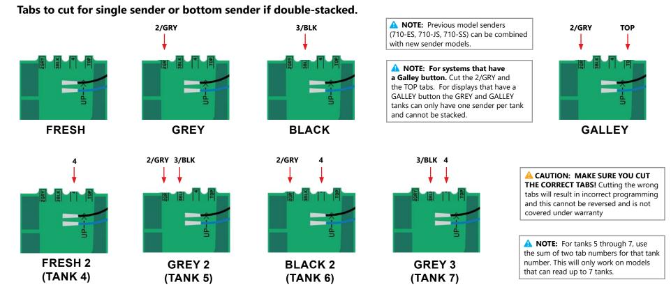
For a double-stacked tank configuration, the top sender requires an additional tab to be cut.
