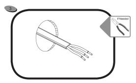
Examine the boats internal wiring. Make sure the wire is in good condition, a clean and bright copper color. If necessary, cut back until the clean wire is found.
