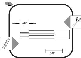
Strip the wire insulation back 5/8". Do not solder the end of the wire.
