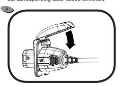
Insert plug into the inlet and press down on the inlet cover.
