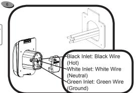
Remove plastic strain relief component from rear of inlet and set aside. Loosen color coded screws.
