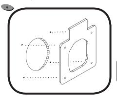
Test your new SmartPlug for proper fit and alignment of screw holes. (On some installations, you may have to modify the hole in your boat to accept the new plug). Pease use the enclosed rear mounting gasket as template if necessary.
