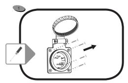
Remove old inlet's four mounting screws and remove the inlet from the boat. If the old inlet has a rear safety enclosure, loosen the strain relief clamp and remove.
