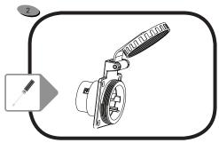
Loosen the screws on the side to disconnect the inlet from the boats internal wiring and remove the old inlet.
