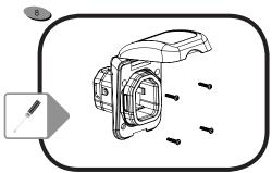
Reposition the new SmartPlug inlet in the \*boat and mount with the four #10 screws (or with the four screws from the old unit).
