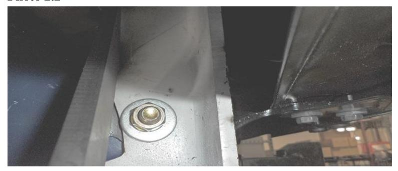
To install the tie down with the SuperHitch Hero #T1300H. Reuse the three fasteners securing the side plate of the hitch to the frame. See Photo below.
