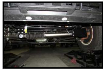
5. Loosely install the tie rod bracket onto the drag link. Loosely install the solenoid end of the TruCenter onto the attachment plate with the 3/4" x 4" bolt supplied in the bracket kit and 3/4" hardware provided in the TruCenter kit.
