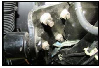
Using a 18MM socket, remove the bolt from the steering stabilizer shock (left). Using a 15MM socket, remove the four (4) u-bolts from the other end of the steering stabilizer shock (right). Set the shock and all hardware aside it will not be reinstalled.
