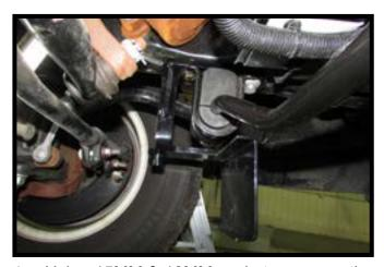
4. Using 15MM & 18MM sockets, remove the two (2) bolts from the DS sway bar. Install the attachment plate in between the sway bar and frame. Reinstall the sway bar with the 10MM hardware provided and fully tighten.
