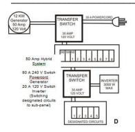
The TS-30 A can be installed between inverter (default) and a circuit panel supplied by a larger amp alternating power supply (dominant).
