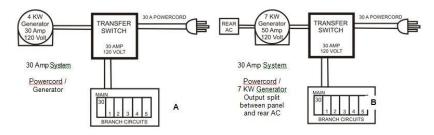
Diagram 1 – Typical Generator Power Cord Connection
