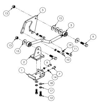
NOTE: There are two (2) axle brackets in this kit. One fits the 110/115 rear axle and one fits the 135/150 rear axle. Match the bracket to the bolt pattern and discard the bracket that does not fit.
