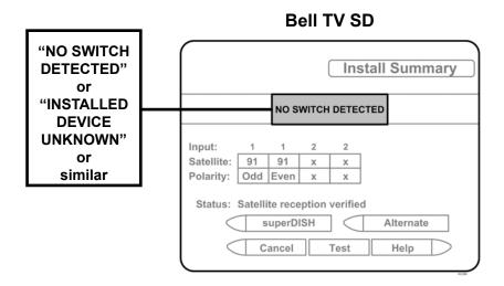
If the indicated results are not obtained, go back to Step 4 and run test again. Contact KING if the check switch fails to load after 4 attempts.
