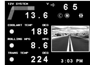
newer required). You should see these update as the transmission shifts. Beside that, the VMS displays the Transmission Mode. The Mode indicates the aggressiveness of the transmission; on most coaches Mode On indicates less aggressive shifting for better fuel economy. The Error icon (an exclamation mark) will appear to indicate problems.
