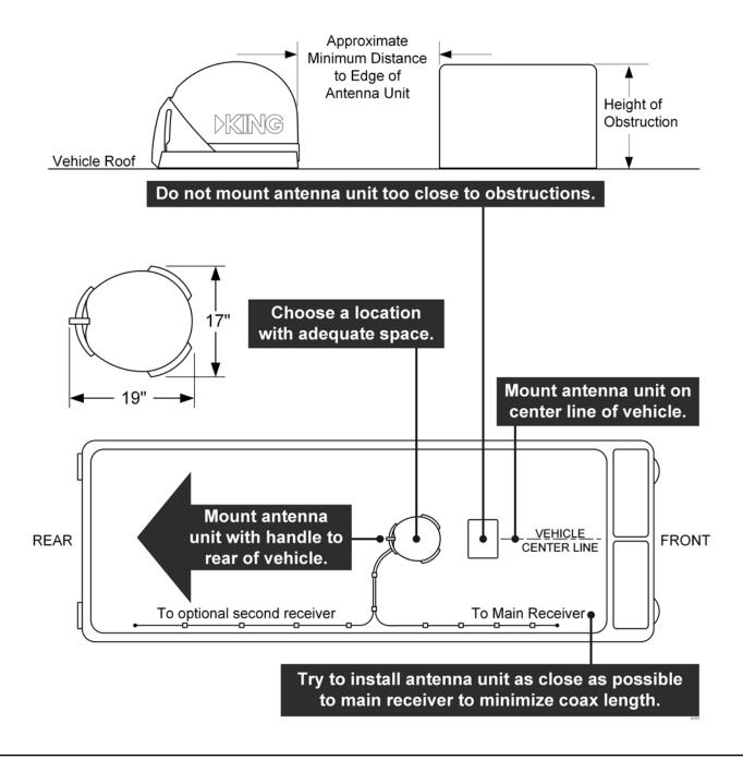
**NOTE:** The installer is responsible for determining the most appropriate fastener to secure the antenna unit to the roof. Depending on the roof material, fasteners such as lag screws, well nuts, sheet metal screws, toggle bolts and T anchors may be used, and should always be used in combination with a roof compatible sealant.
