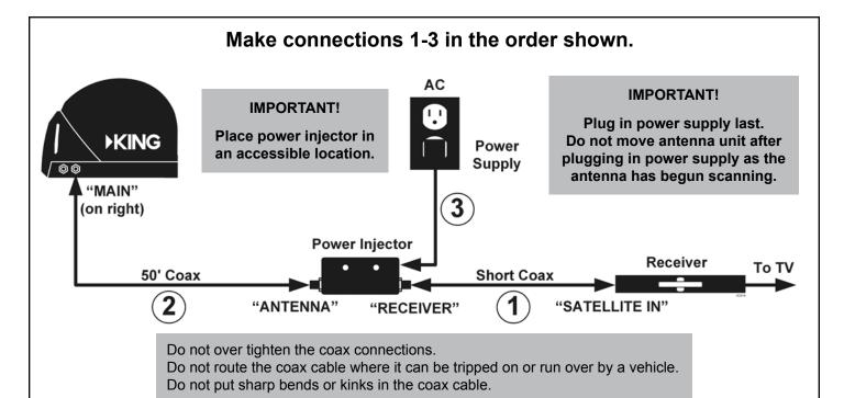
When all connections are made, the antenna unit will scan for the DIRECTV 101 satellite.
