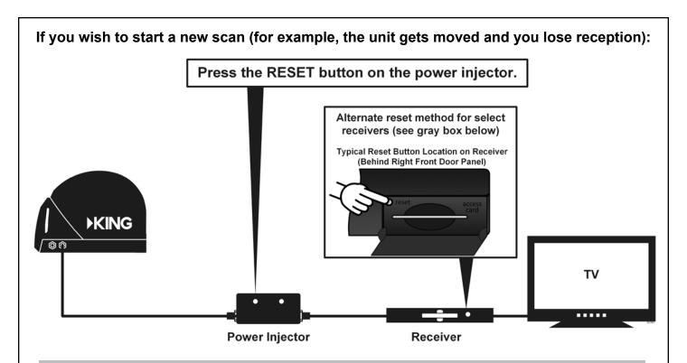
Pressing the power injector's RESET button is the preferred method to start a new scan, but there are two alternate methods as well:
