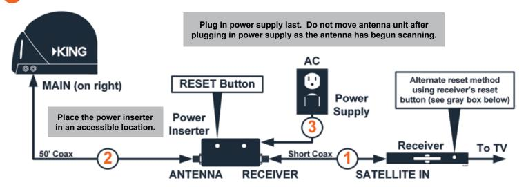
Do not overtighten the coax connections. Do not put sharp bends or kinks in the coax cable. Do not route the coax cable where it can be tripped on or run over by a vehicle.
