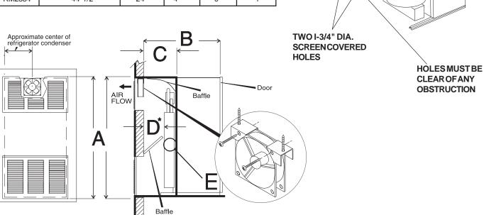
\* When dimension "D" exceeds 1", it is necessary to add baffle (E) above lower access vent, as shown, for more efficient operation in warm temperatures.
