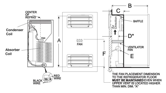
When dimension "D" exceeds 1", it is necessary to add baffle (E) above lower access vent, as shown, for more efficient operation in warm temperatures.
