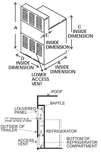
**Note:** B, C & D inside dimensions are minimum installed dimensions as zero clearance is required.
