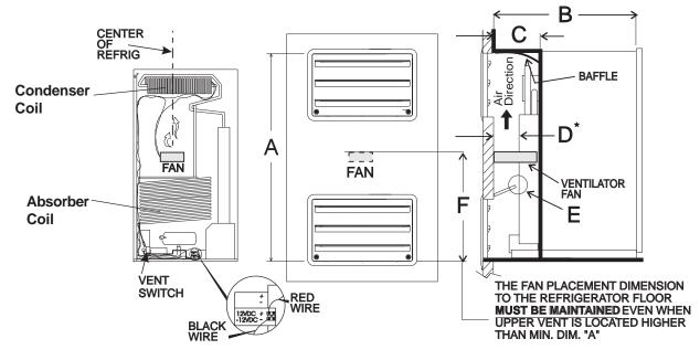
\* When dimension "D" exceeds 1", it is necessary to add baffle (E) above lower access vent, as shown, for more efficient operation in warm temperatures.
