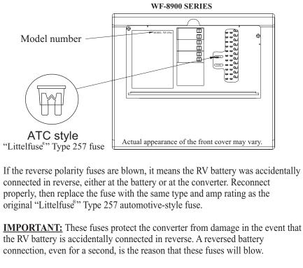
The fuse rating that the manufacturer suggests for the output fuses will be marked on the unit. Replace only with same type and rating.
