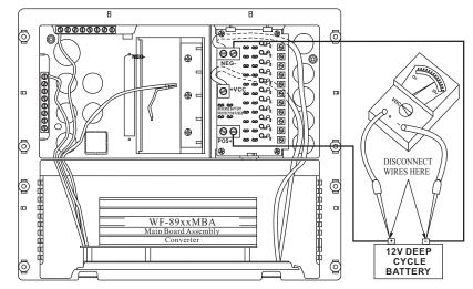
If the converter output voltage at the battery reads in the 0.0 Vdc range, or the battery is not charging, check for:
