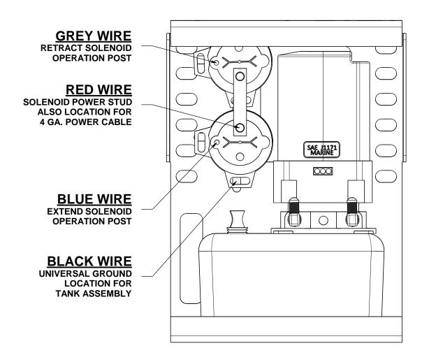
HARNESS WILL COME WITH NECASSARY WIRE CONNECTORS AT EACH END AND WILL BE PREVIOUSLY ATTACHED TO THE RECEIVER CONTROL PAD.
