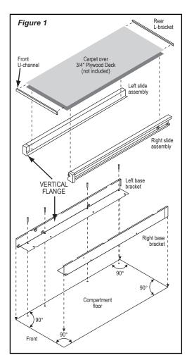
**5.**□ Attach the front U-channel and rear L-bracket to the deck using pan-head screws and the holes provided. The 2-way pull SuperSlides use U-channel on front and rear.
