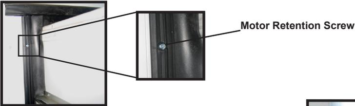
Locate and remove motor retention screw located near top of each vertical column.
