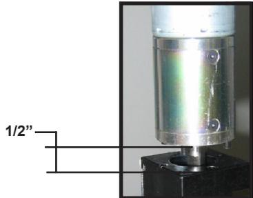
Pull the motor up until disengaged, about 1/2"
