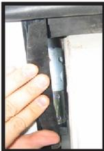
Bend back wipe seal and visually locate motor
