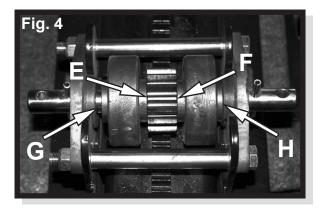
LCI recommends Mobil One Fully Synthetic 10W-30 Motor Oil to lubricate gear pack.
