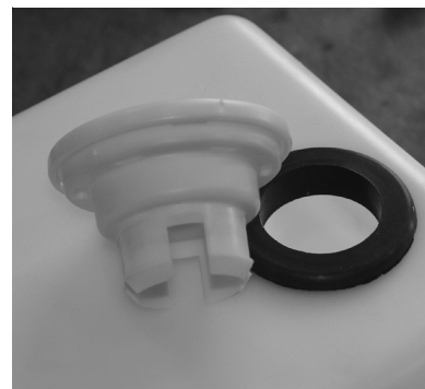
6. FILL CAP-FILL RESERVOIR TO WITHIN 1/2" FROM THE TOP WITH SLIDEOUT FULLY RETRACTED
