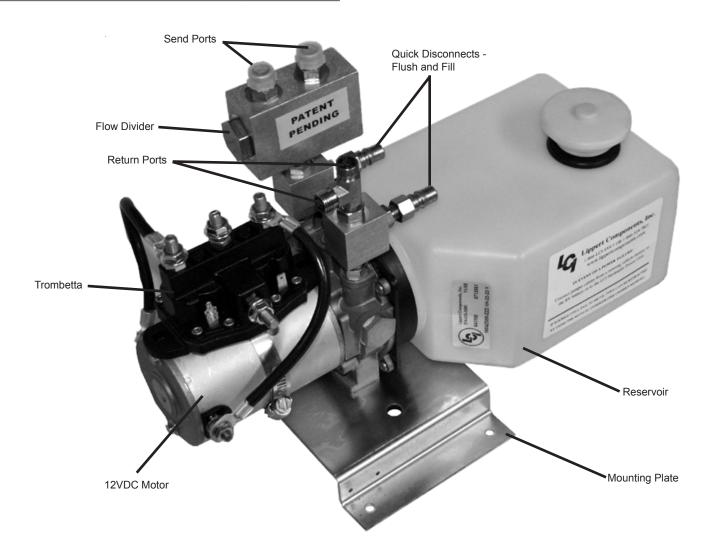
Send ports for the extention of the Full Wall Slideout System are positioned on the block with the Flow Divider. The return ports are positioned on the small square block on the retract side of the pump unit.
