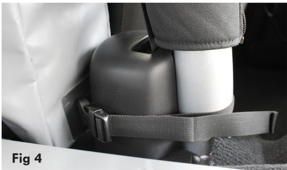
3-Buckle the E strap around the rear vertical roll bar, above the seat belt holder, without twisting the strap (Fig 3 and Fig 5).
