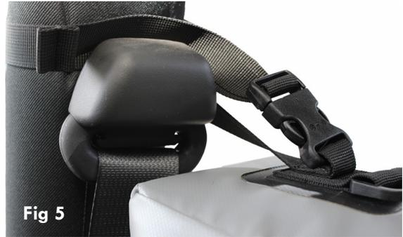
4-Buckle the F strap around the front vertical roll bar, above the seat belt holder, without twisting the strap (Fig 3 and Fig 6).
