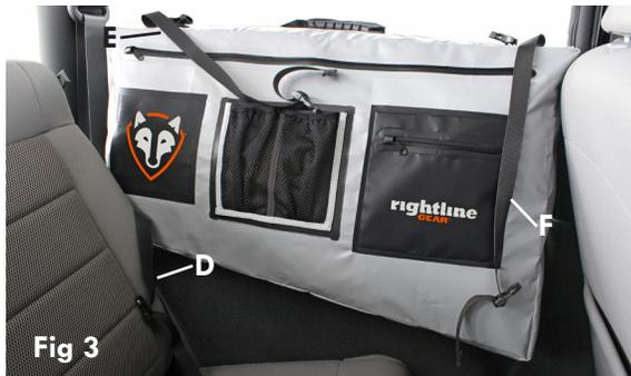
2-Buckle the D strap around the base of the rear vertical roll bar, without twisting the strap (Fig 3 and Fig 4).
