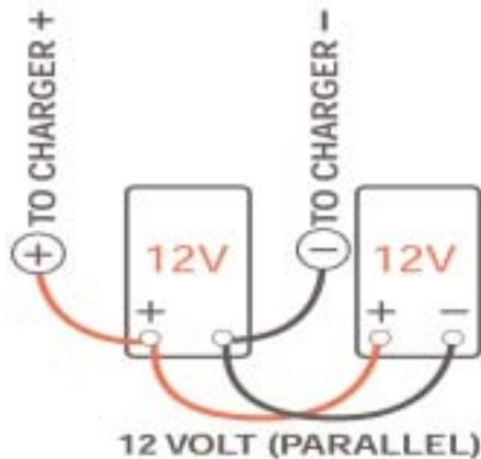
Connect each battery to one another using 18 gauge (lamp cord type) insulated wire. Strip at the points where you wish it to be in electrical contact with the posts of each battery, then use ring or clip connectors. VDC Electronics, Inc. does not provide any type of wire harness to accomplish this, due to the many variations in size and terminal configuration.
