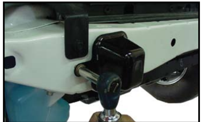
8. Remove both tin covers on front of bumper to allow access for nut strip.
