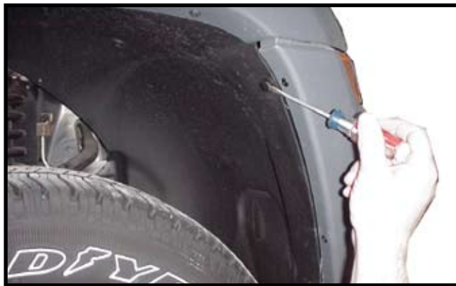
4. Remove three plastic push fasteners from each wheel well.
