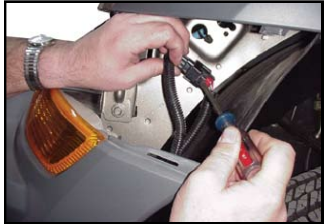
7. Unplug front fascia wiring on each side (slide red lock back, then release).
