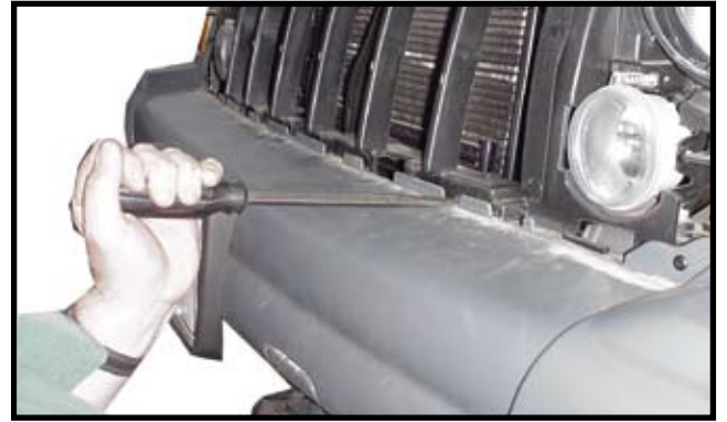
6. Release plastic clips and remove fascia.
