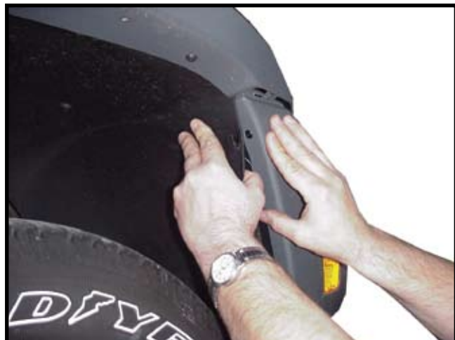
5. Push fascia in to release clip on each side.
