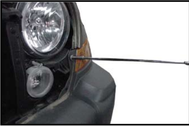
2. Remove two bolts from fascia by head lights.
