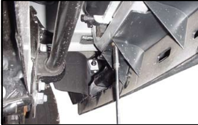
3. Remove two bolts from bottom of fascia behind air dam.
