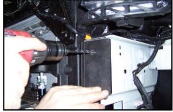
**16.** Using base plate as template, drill a 5/16" hole into end of frame, install 3/8" self-tapping bolt on each side and tighten. Remove Clamps.
