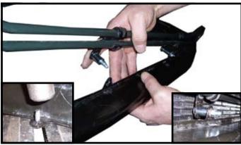
remove cooler line studs in a vise, then drill out holes to 1/4". Fasten tin support with one washer and nut previously removed on top to one side and leave it loose. Install cooler lines by using plated spacer bushings, 1/4" x 1-1/2" bolts, lockwashers, and nuts. Finish installing lower tin support and tighten. Adjust lines for clearance thru oval hole in baseplate, lines cannot rub on baseplate. Rubber hose may be needed for protection (not included).
