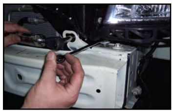
18. Reinstall bumper with the remaining bumper bolts. Note: Top bumper mounting tab must lay flat on frame. If not, bottom tab was not bent flat enough or cut off far enough. If ECO use stud factory stud to fasten shutters and bumper. Plug in shutters.
