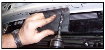
21. Drill 3/8" holes into bottom of bumper using baseplate center support bracket as template. Install 3/8" x 1-1/2" bolts, 3/8" lock washers and 3/8" nuts on inside of bumper and tighten.
