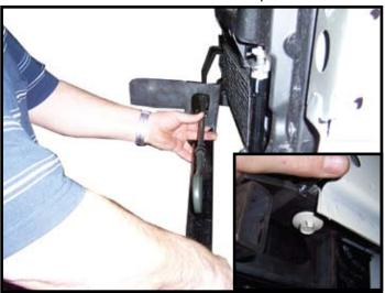
15. With an assistant, slide cooler line carefully thru side hole of baseplate on passenger side. Lift baseplate up into place and clamp to bumper mount. Install previously removed bottom bumper bolts and tighten. If ECO have shutter system behind baseplate when installing and put bottom mount in. NOTE: Use LOCTITE. Blue on all bolts during installation
