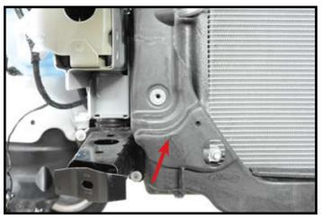
**14.** Remove the plastic push fastener from the bottom of passenger side air deflector and drill hole 2" to the left of factory hole and reinstall air deflector fastener. Be careful to not drill into hoses behind plastic.
