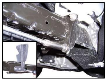
5. IF EQUIPPED Remove two nuts that hold cooler line to lower tin support. Remove lower tin support, three nuts and washers on each side. Remove both filler panels from tin support. (These will not be reused)
