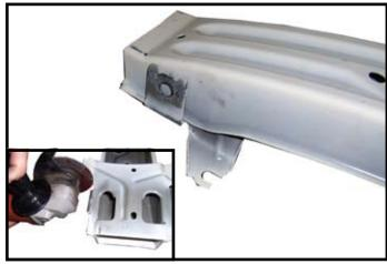
**17.** Before installing bumper, first bend down lower mounting tabs flat or remove completely. Grind bumper as shown, approximately 1/4".
