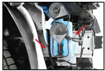
8. Remove two screws from washer tank and pull out of way so bracket and bolts can be installed on passenger side. NOTE: Four push fasteners from inner wheel well may be removed to make installation easier or remove tank completely.
