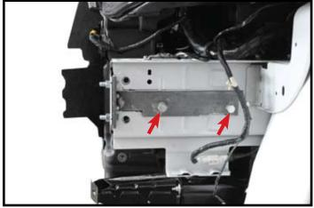
7. Install driver side bracket with 7/16" x 1-1/2" bolt, lock washer, and flat washer with nutstrips using hole in from of frame exposed when bumper was removed. NOTE: Use LOCTITE. Blue on all bolts during installation
