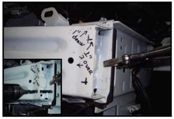
19. Mark out front of bumper for drilling 1" from the top and 2-5/8" centers and 1/2" from outside edge. Drill two 3/8" holes thru bumper, baseplate, and frame on both sides. Fasten with 3/8" x 1-1/2" bolts, 3/8" lock washers, and 3/8" hex nuts. **Note:** Some models are equipped with a hardened steel bumper and can not be drilled easily so grind a 3/8" slot where the holes are and mark and drill holes on the baseplate accordingly. Holes should match up to previously installed brackets.
