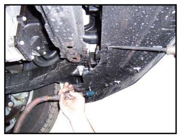
Remove three plastic push fasteners and four screws from bottom of facia.
