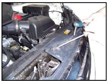
1. Open hood and remove four plastic fasteners and two bolts from top of facia.
