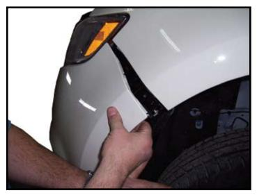
Unhook fog lights, if equipped, side marker lights and remove facia by pulling straight out by fender, then pull off.
