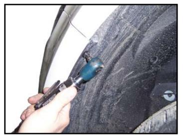
Remove three screws from wheel well to fender on each side.
