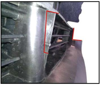
**12.** Trim as shown in picture on both sides for clearance of baseplate crossmember.
