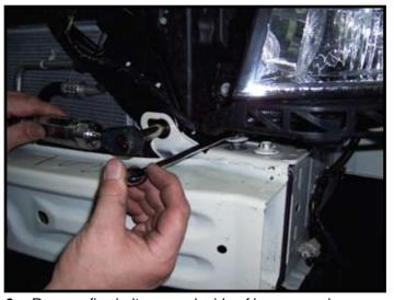
6. Remove five bolts on each side of bumper and remove bumper. For late model Edge's with ECO remove two nuts from outer edge of shutter system, unplug wires, and release mount on bottom center of shutters. Then remove three bolts and one stud from bumper and remove bumper.
