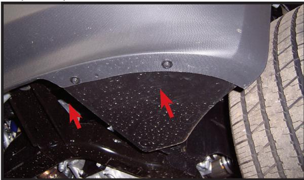
3. Remove two screws from the bottom of the fascia on each side. Pull out firmly on outer corner of fascia from the front of the fender. Unplug fog lights if equipped.
