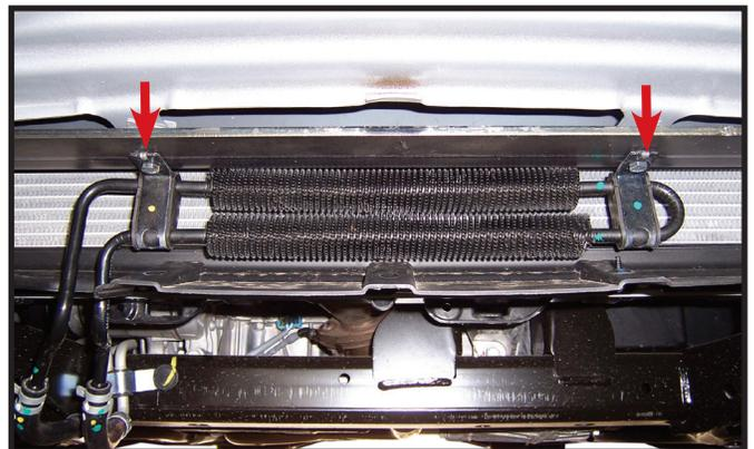
28. **If Equipped** Using the 1/4" x 1 bolts with flat washer and lock washers replace the cooler mounting it to the baseplate in the holes provided as shown.
