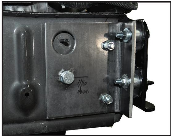
24. Using the supplied fish wire, fish the 3/8" serrated flange bolts up through the hole in the bottom of the frame as was done with the nutstrip. Fasten the bolts in place using 3/8" lock washers and 3/8" nuts. NOTE: Use blue on all bolts and tighten all bolts according to chart on front page.
