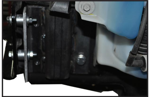
26. Install the driver side bracket in the same ways as on the passenger side. Follow step 21-24 for order of how to install bracket.
