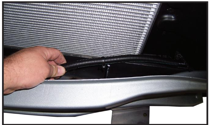
27. Route wiring as desired to prevent damage from harness
