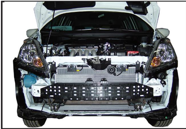
11. With an assistant install baseplate with bumper over top of baseplate onto vehicle re-using the eight bolts removed in step 6. Use blue **LOCTITE** on all bolts and tighten all bolts according to chart on front page.
