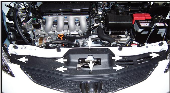
1. Open hood and remove 8 plastic push fasteners from top of grill.
