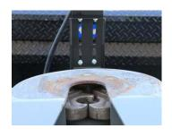
Fig. 3 F CAUTION! – Bracket must be centered with king pin slot of hitch, and must be square and level with the hitch ware plate. Fig 3.
