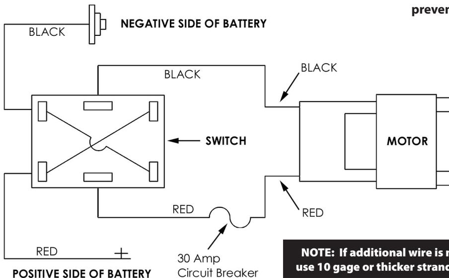
**NOTE: If additional wire is needed, use 10 gage or thicker stranded wire.**
