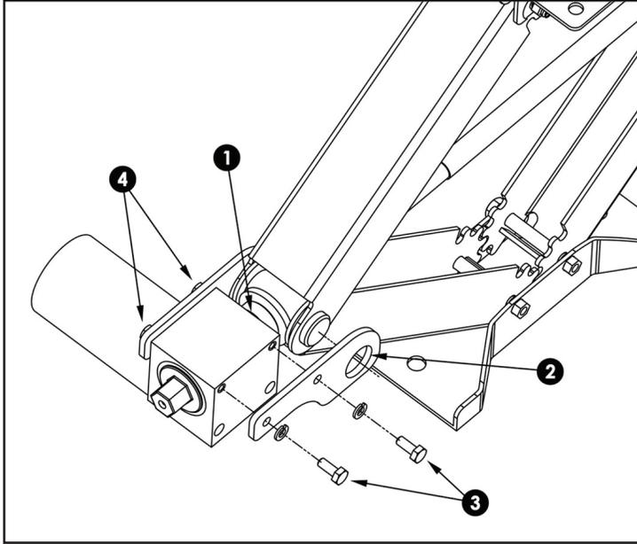
1. Slide motor onto the hex head of the jack's drive screw.
