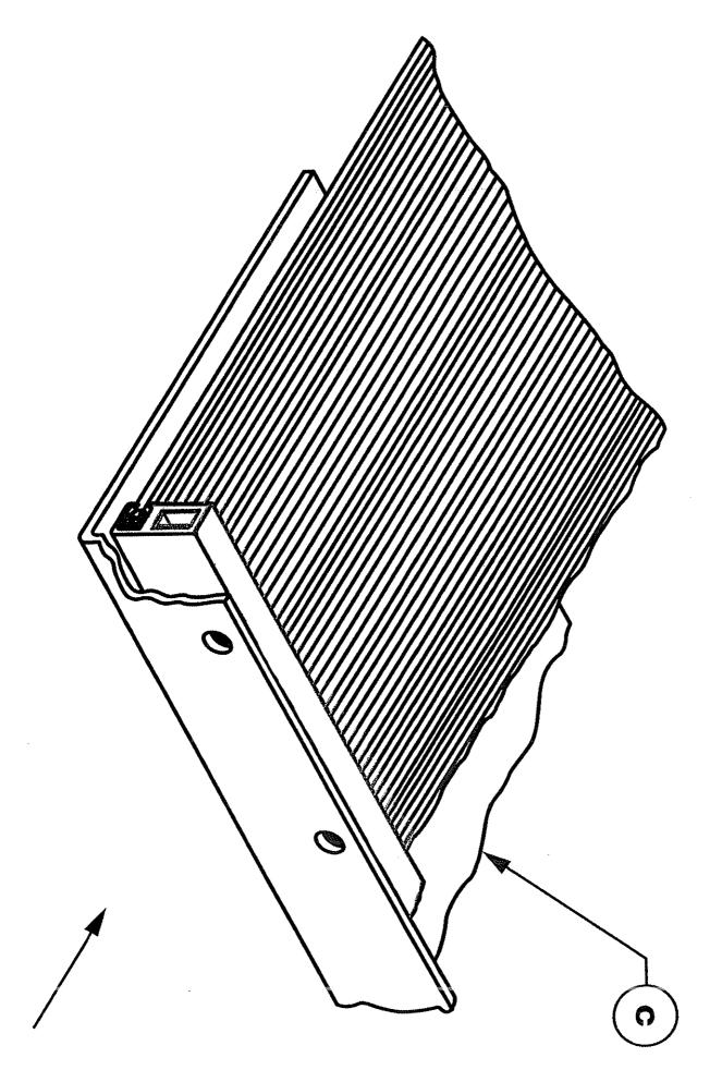
4) ALIGN HOLES AND INSERT 1 EA FLAT WASHER NUTS AT THIS TIME). THRU HOLES OF ALL ITEMS (DO NOT INSTALL LOCK ONTO BOLT AND INSTALL 9 BOLTS W/ WASHERS,
