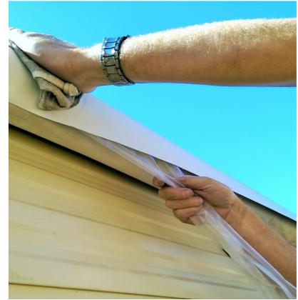
Now with the Awning Guard in place along the RV-Awning seam.
