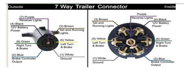
To wire the Brute jack through a 7way plug instead of wiring to the trailer battery - take the black wire off the jack and wire into the black terminal of the 7way plug, then run a ground wire from the white terminal of the 7way plug to one of the mounting bolts used to secure the jack to the trailer with a ring terminal. The jack will only work while the 7way plug is still connected to the 7 way plug on the vehicle.
