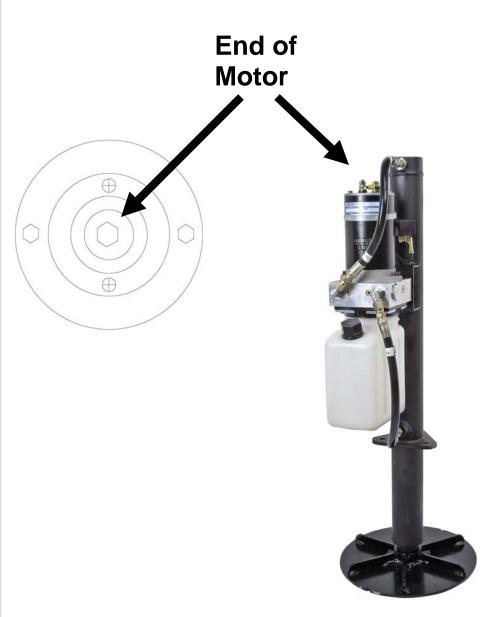
Override Coupler (Under Foil Seal) Accepts 6mm (1/4") Hex Key
