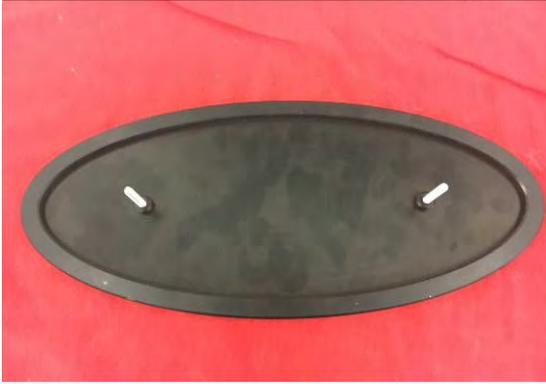
6. Insert threaded studs into the back of larger front emblem.
