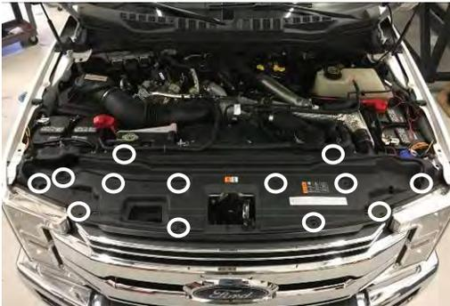
2. Remove plastic cover by removing 13 retaining clips (number of retaining clips may vary) with flat head screw driver (locations shown above).
