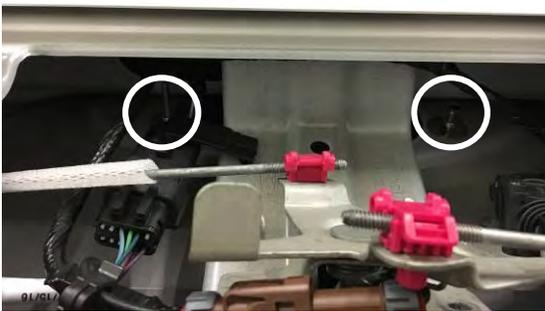
7. While holding emblem in place use the rest of supplied hardware to secure emblem from inside tailgate as shown above.
