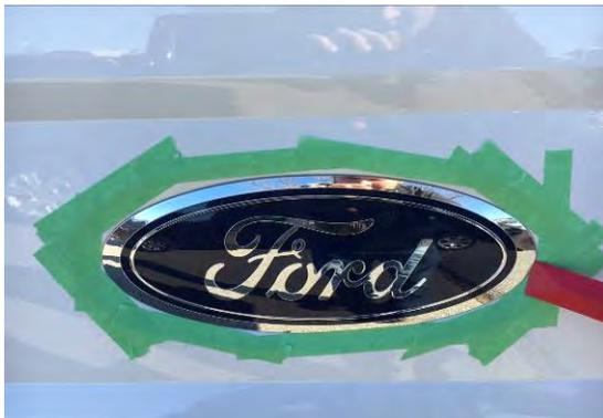
1. Pry off factory rear emblem with a plastic pry bar. Be very careful not to damage the paint. Tape can be used to protect paint. There a 4 plastic clips and tape that hold emblem on.
