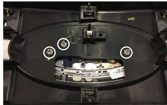
5. Remove grille. Once grille is removed, Lay grille on flat surface (Protect grille front face) remove 3 10mm nuts to release front emblem. (locations shown above)
