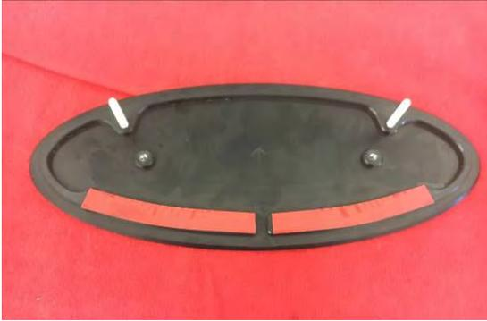
5. Insert supplied threaded studs to upper holes on smaller rear emblem. Lower threaded holes are not used.
