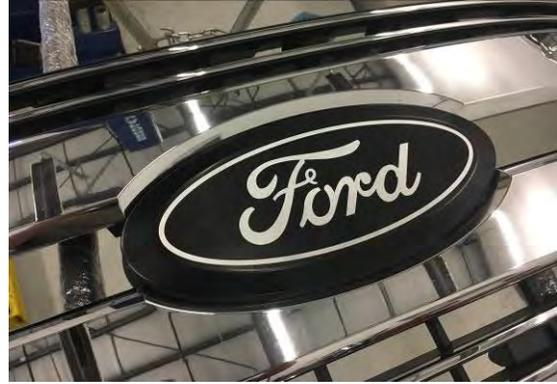
7. Slide emblem through holes in grille and mount using the rest of the supplied hardware. Use 3/8" wrench to tighten hardware. Reinsert grille and it's components.
