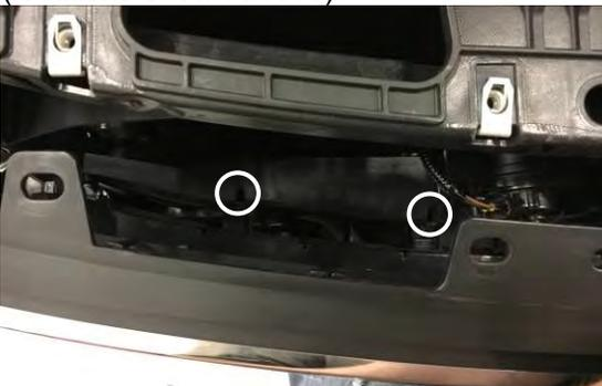
4. Pull upper grille forward to release upper grille clips. Once out, release 4 bottom clips with a flat head screwdriver. Passenger side locations are shown. Repeat on driver side
