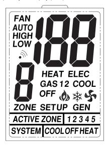
The LCD display screen is the main interface between the user and the thermostat. This will display which zone the user is looking at. When the system is first powered up, the thermostat determines how many zones are connected to the system and only displays the zones detected.
