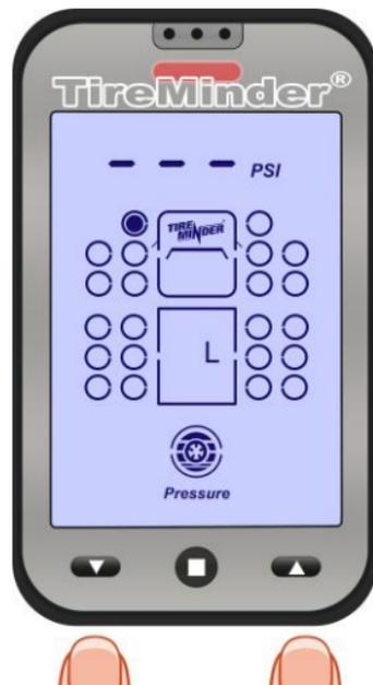
Using the **right or left buttons**, move to the next tire position you wish to monitor. Again you will have a red light which will turn green. Repeat this procedure until you have installed all the transmitters.
