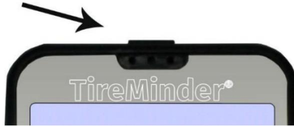
If the unit does not light up immediately, simply plug it into a live 12 volt power outlet using the cigarette lighter adaptor or the USB cable to any USB port. You may work with the unit while it is charging or after 15 to 20 minutes it will have sufficient power to do a complete installation without it being plugged in.
