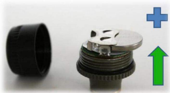
The cover should only be finger tight (*snug*) so as to remain waterproof. Please, DO NOT use pliers and a pipe wrench! Over tightening will damage the “O” ring.
