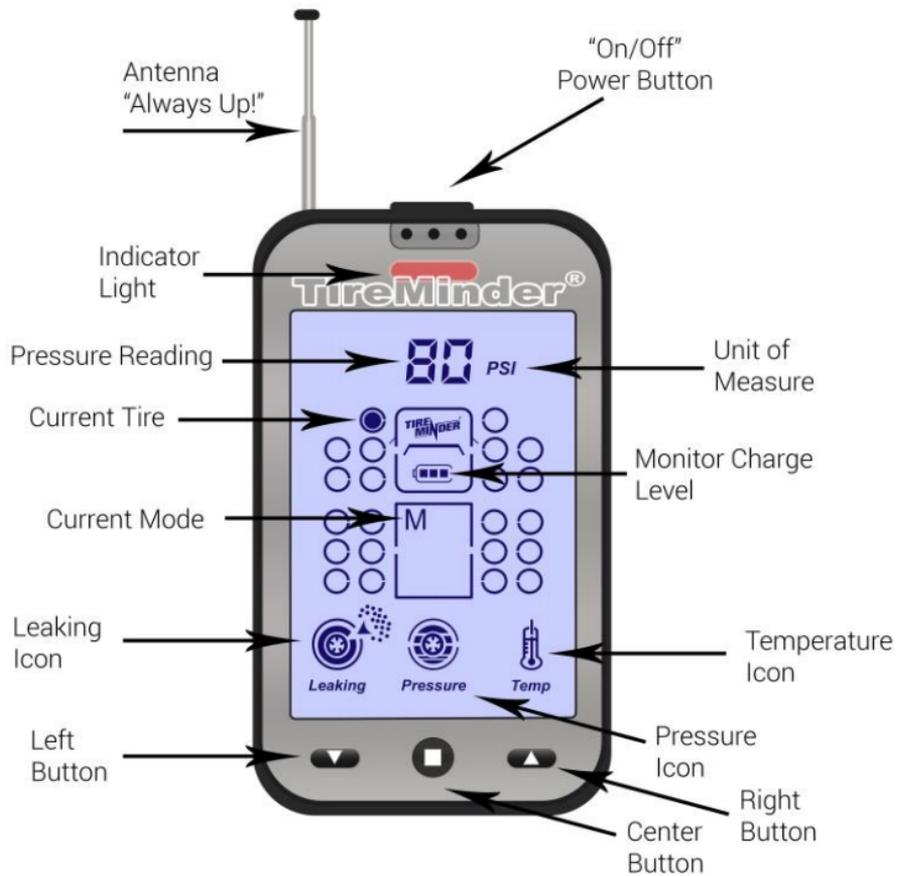
The TireMinder® TM-A1A™ Tire Pressure Monitoring System (*TPMS*) allows for constant monitoring of a vehicle's Tire Pressure & Temperature. The system can receive wireless information from up to 22 wheels. Various levels of warnings are issued for pressure changes (*under & over*), high temperatures and low battery status.
