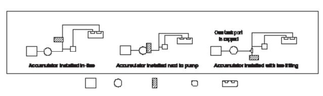
The RACT820-JG has 2 John Guest 3/8" push connect fittings. This tank can only be mounted with through connections. See diagrams in figure 2.
