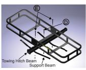
Position the towing hitch beam underneath the cargo baskets, with the caution sticker facing away from the hitch pin holes. Lightly fasten the hitch beam to the cargo baskets using Bolt Assembly D in the center bolt hole. Bolt Assembly D consists of (1) 3/8" x 31/2" long bolt, (2) 3/8" Flat Washers, and (1) 3/8" Nut.
