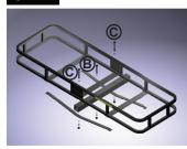
Note: If you have a towing option, skip to the Towing Option Instructions below. Position the hitch beam underneath the cargo baskets, with the caution sticker facing away from the hitch pin holes (i.e. away from the vehicle). Lightly fasten the hitch beam to the cargo baskets using Bolt Assembly B in the center bolt hole. Bolt Assembly B consists of (1) M10 x 80 Bolt, (2) M10 Flat Washers, (1) M10 Lock Washer, and (1) M6 Nut.
