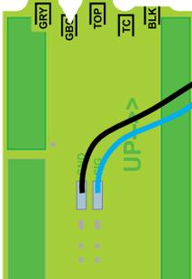
Example of corrected FRESH SINGLE or BOTTOM sender programming (TOP tab cut by mistake)
