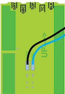
Example of corrected GREY SINGLE or BOTTOM sender programming (BLK tab cut by mistake)
